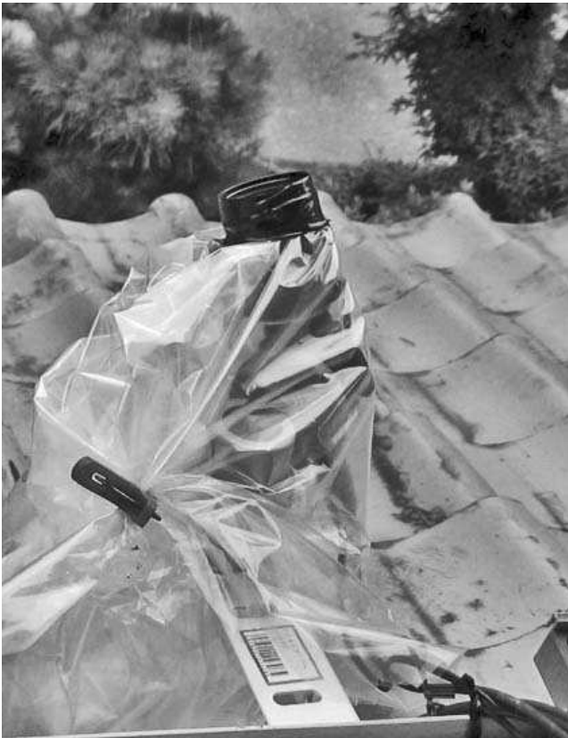
Figure 2 – CCD observation view. Easy vinyl sheet protects a camera and makes it possible to place it outdoors.
