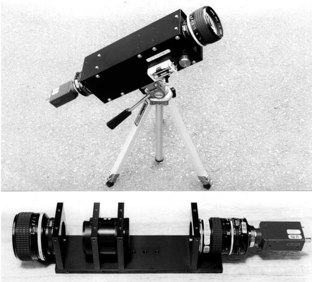
Figure 1 – Image-Intensifier set (top) and its inside view (bottom). The equipment consists of camera, lens, image-intensifier, close up lens and CCD video camera.
